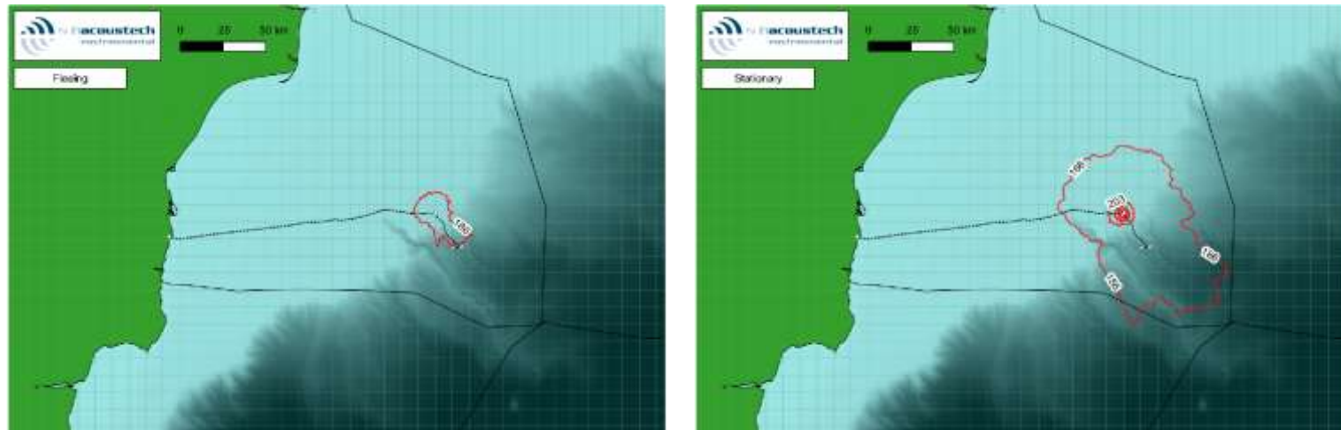
Figure 5-15 Noise plots showing the predicted unweighted SEL_{cum} zones fish of impact (Popper et al., 2014) from impact piling at the open water modelling location for the MENCK 800S hammer upper bound scenario for four sequentially installed piles, contours are TTS (outer), \geq 203 dB (inner)
