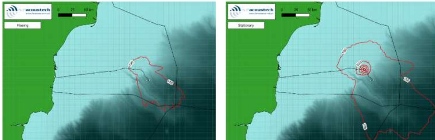
Figure 5-23 Noise plots showing the predicted unweighted SEL_{cum} zones of fish impact (Popper et al., 2014) from impact piling at the open water modelling location for the MENCK 3200iS hammer upper bound scenario for four sequentially installed piles, contours are TTS (outer), \geq 203 dB (inner)
